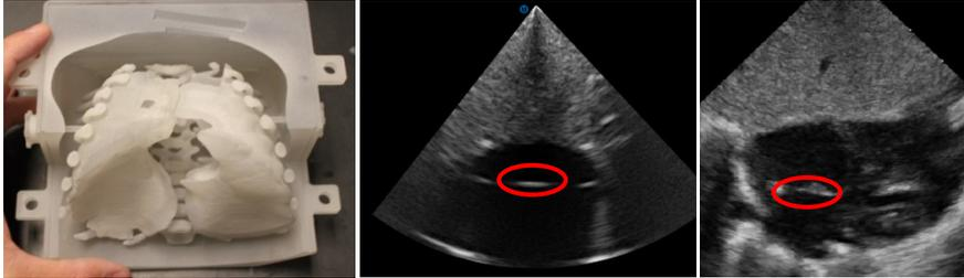
Image to the left represents a 3D printed replica of an infant torso generated from anatomic data. The middle image is the ultrasound image through this manikin once filled with tissue mimicking media. The image to the right is an ultrasound image of a human neonatal atrial septum which shows how similar the artificial replica mimics the human condition.
